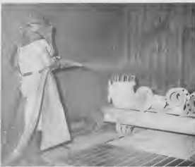
BLASTER AT work in new Dry-Blast Cleaning Facility in Shop. 'BLASTER' TRAHANDO den e facilidad nobo pa limpia metal.
